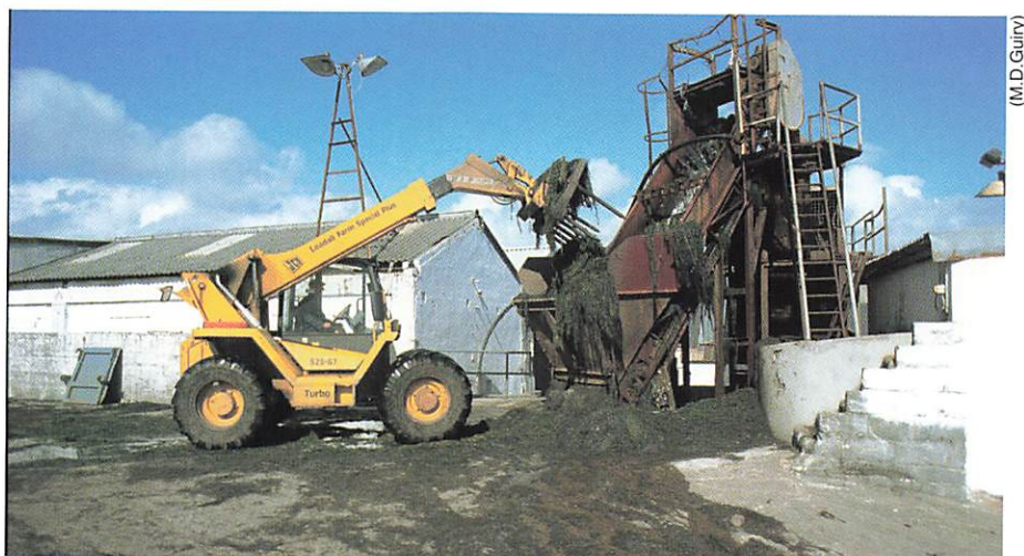
Fig. 20 Freshly harvested, wet Ascophyllum nodosum being loaded into a hopper at Arramara Teoranta's Kilkieran factory in Co. Galway, for processing into seaweed meal. Primary processing into seaweed meal consists of washing, mincing, kiln drying and sieving into different grades of meal. The resultant seaweed meal is either used as soil conditioner/fertiliser, animal fodder supplement, liquid seaweed extract or transported to Scotland for alginate production.
